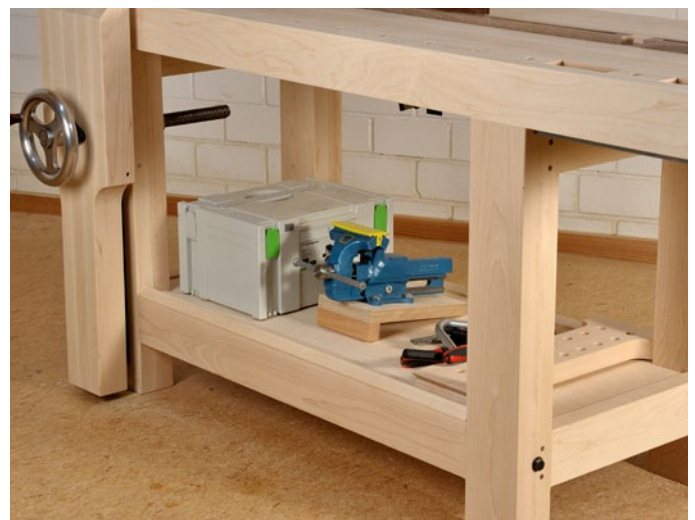
The deadman can also be removed and, along with any other tools, be stored on the large shelf supported by the rails joining the base of the legs.
