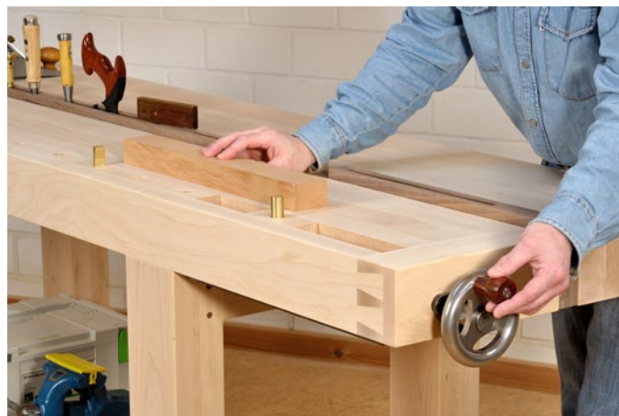
Longer and thicker workpieces can be clamped to the bench top using round brass bench dogs.
