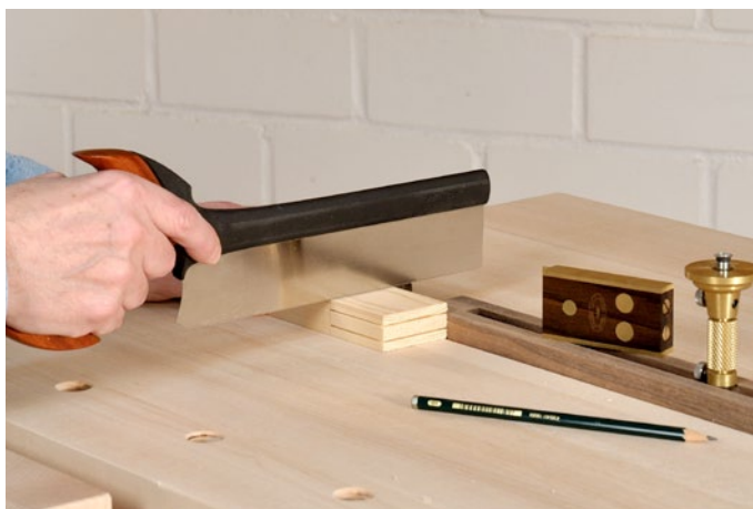
Because the board stands 15 mm proud of the bench top, it can also be used as a saw stop, while cutting the shoulders of a tenon, for instance.
