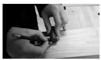
Thread the barrel nut onto the bolt so the bolt protrudes about ¼" past the nut, and while holding the bolt in the correct place for your leg width, mark the center of the barrel nut on the bolt line.
