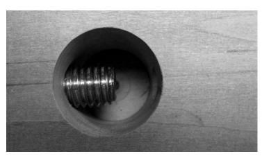
The bolt should end up right in the center of the barrel nut hole.
