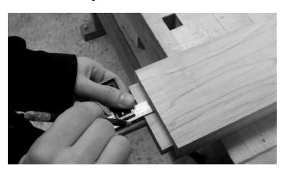
To find the position of the barrel nut hole, you're going to use the position of the hole you just drilled as a guide.
