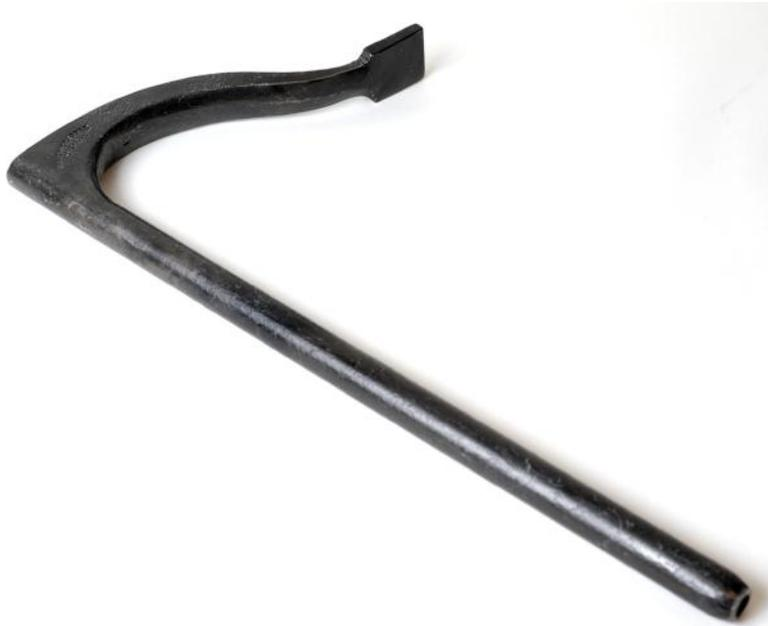
Thanks for purchasing the Benchcrafted Hand-Forged Holdfast. Our holdfast is based on a French example from the late 19<sup>th</sup> century. It's designed to work in 1" holes in workbenches from 3" to 6" thick.
